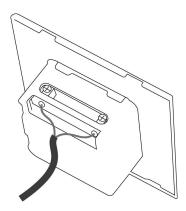
4. To put the back cover on the electrical box and fix it with the screw.
