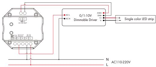
Note: 1. We recommend the number of LED drivers connected to 0/1-10V dimmer does not exceed 100 pieces, The maximum length of the wires from dimmer to LED driver should be no more than 50 meters.
