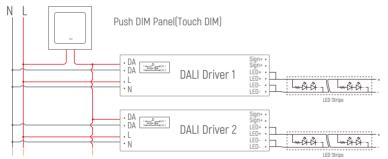
Remark: Only use open push button without indicator light. Maximum cable length between each Unit: 20 meters.
